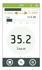
During a measurement, the mobile app shows the measurement start time ( $\stackrel{\frown}{\square}$ ) and the measurement duration time ( $\stackrel{\frown}{\square}$ ).
