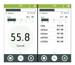
**Total** displays instantaneous parameters and parameters that are calculated for the total measurement time. It is the main display for single measurements. SLM view (left) shows an instantaneous broadband parameter (bar graph) and one calculated broadband parameter. List view (right) shows an instantaneous broadband parameter (bar graph) and a list of calculated broadband parameters. Each view contains a unique bar graph.
