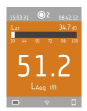
In the middle is the measurement display. There are views for broadband parameters (SLM view and List view) and a view for information about your data (About data view).
